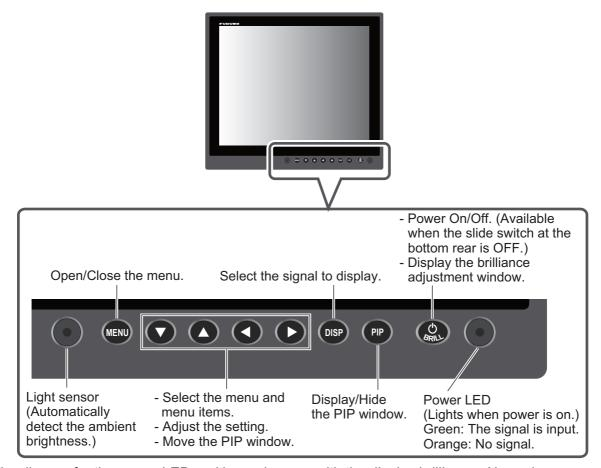
The dimmer for the power LED and keys changes with the display brilliance. Also, when you connect the monitor unit to FAR-21x7, FEA-2107 or FCR-21x7, the dimmer for the power LED and keys changes with the brilliance modes (Day, Dusk, Night) of those models. When you connect the monitor unit to the equipment other than FAR-21x7, FEA-2107 or FCR-21x7, the control is done from the MU-190. If the keys of MU-190 are not illuminated, provide external, dimmable illumination, e.g. gooseneck lamp.
